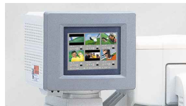
The digital monitor displays positive images of the negatives as well as error messages and instructions.
