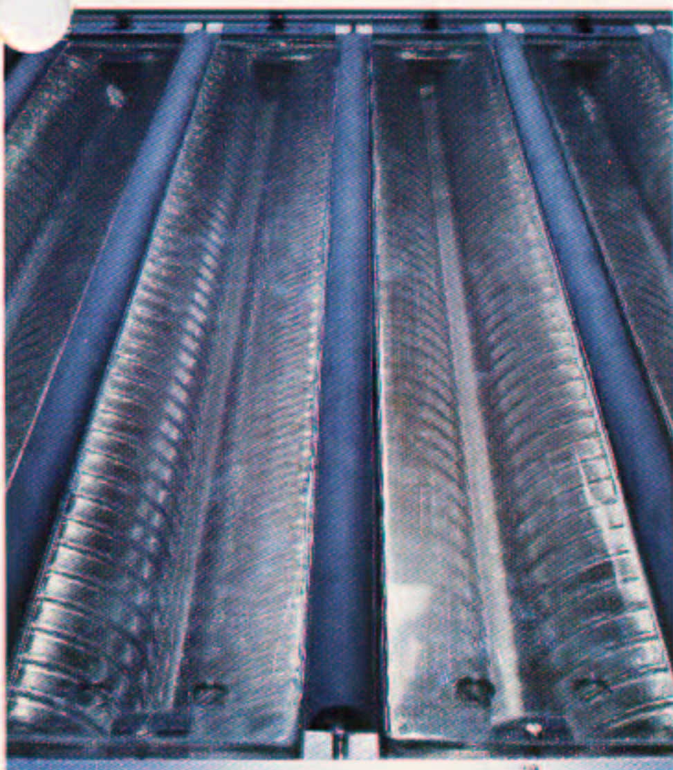
Self cleaning crossovers, and sealed tanks.
