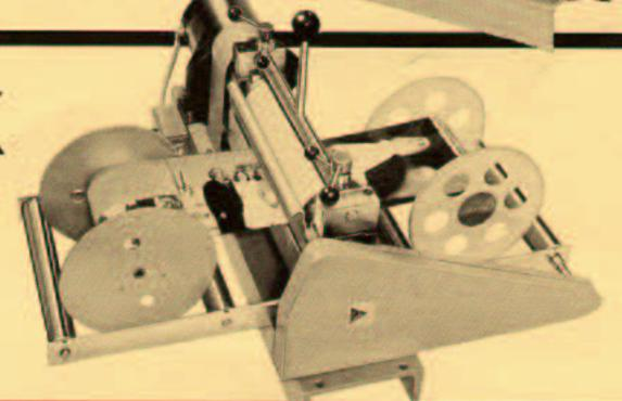
for prints in standard rolls up to 11" width. Speed: 25' per minute; Rugged 1/2 h.p. gearhead motor: 120V, 60c, AC.
